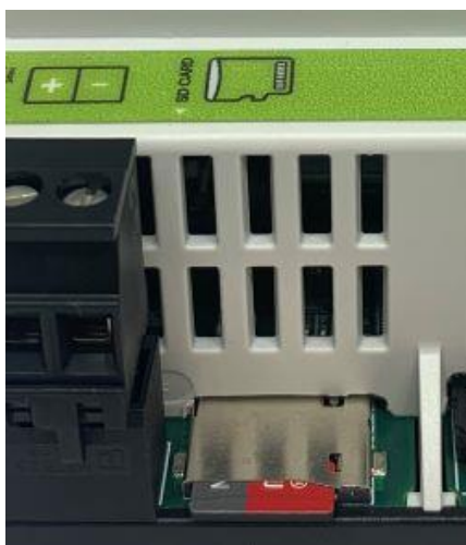
Fig.1 SD Card insert
