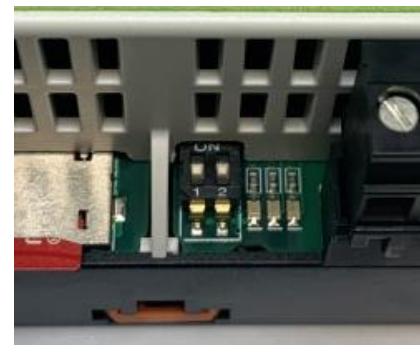
Fig. 6 Example DIP-SWITCH OFF position
