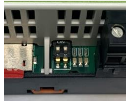
Fig. 6 Example of DIP SWITCH position: OFF OFF
